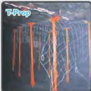
T-Prop Easy to install to 30Kn at the work face and is a mechanical temporary support prop. The unit is modular and is refurbishable with cost effective results.
