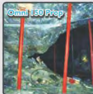
Omni 150 Prop Provides up to 190Kn load and 300Kn dynamic load at 3meters/sec. Can be used as permanent or re-usable support and is a blast on prop. Props can be used with set pieces in bad areas for arch support. Supplied in 20, 40 Ton load capacity.
