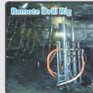
Remote Drill Rig Operated from a safe distance, the rig is easy to use and is low maintenance. Supplied in either double or single stingers with an extension piece fitted for variable heights.
