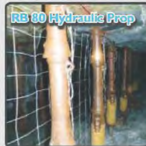
RB 80 Hydraulic Prop Are installed as a blast on prop close to the stope face. Installation loads at 170Kn with slow load resistance at 200Kn and dynamic load resistance of 430Kn at 3meters/sec.
