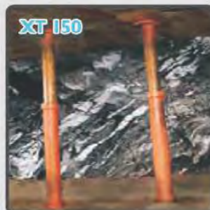
XT 150 Is a yielding friction prop. Installed at 190Kn load and 300Kn dynamic load at 3meters/sec. The prop is a sacrificial blast on prop and can be used with set pieces in bad areas as arch support.
