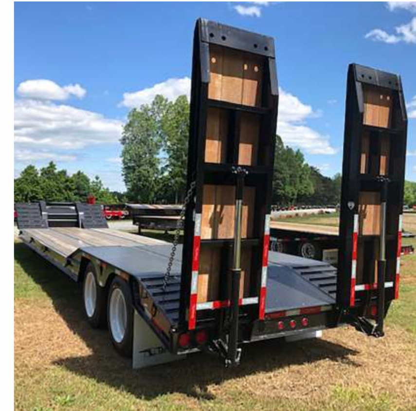
The Talbert 35FG-BVTL's 36-inch sloping beavertail features a 14.98-degree load angle coupled with full-width plate with traction bars outside the main beams for optimal rear loading.
